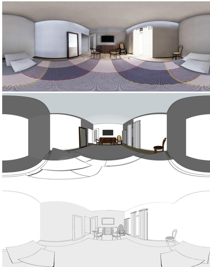
Fig. 4. 360 ° images construction from 3D model, usable for different simplification levels.
